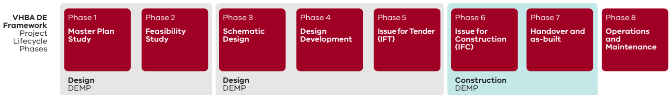
Figure 11: Design and construction DEMP templates aligned to project lifecycle phases for traditional procurement
